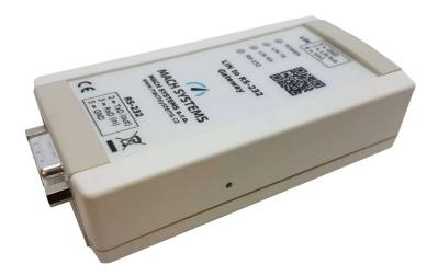
The LIN to CAN and LIN to RS-232 Gateways can be used to interface a LIN bus to CAN or RS-232 respectively. The converters can act as both LIN Master and Slave. A typical use-case is to control or monitor a LIN bus from a PLC with RS-232 port over the gateway device, or simply to bridge a LIN network to a CAN bus.
