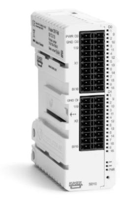
Kvaser DIN Rail S010-X10 Digital is an optional add-on module to the Kvaser DIN Rail SE400S-X10 base module\* with 16 digital inputs and 16 digital outputs. This IP20-rated module is thermal, reverse-polarity protected and surge power supply protected. A power LED displays the state of the module, whilst there are separate LEDs for each of the inputs and outputs.
