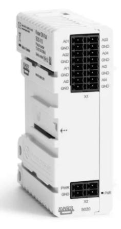
Kvaser DIN Rail S020-X10 Analog is an optional add-on module to the Kvaser DIN Rail SE400S-X10 base module. With four analog inputs and four outputs, this IP20-rated module is thermal, reverse-polarity protected and surge power supply protected. The input voltage range is fixed (between 0 and 10V), and resolution is 12 bits. A power LED displays the state of the module.
