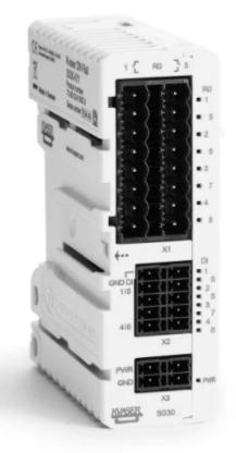
Kvaser DIN Rail S030-X11 Relay is an optional add-on module to the Kvaser DIN Rail SE400S-X10 base module with eight N.O. (Normally Open) relays and eight digital inputs that can be used separately. This IP20-rated module is thermal, reverse-polarity protected and surge power supply protected. A power LED displays the state of the module, whilst there are separate LEDs for each of the digital inputs.
